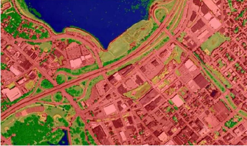
Aerial photography of downtown Portland, ME, classified into open space (greens), impervious surfaces (pink), and water (blue)
